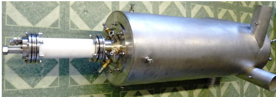
Fig.13. Photograph of a plasma-assisted gasifier for contaminated liquid hydrocarbon destruction.
