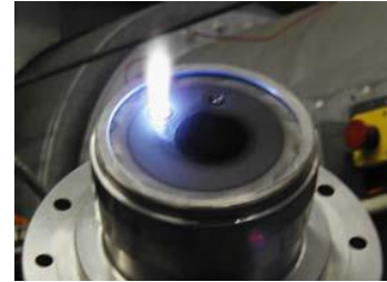
Fig. 2. Photograph of a DC plasma igniter in operation, after Matveev et al [48, 62].
