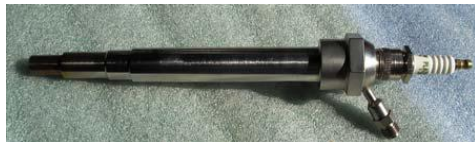
Fig. 3. Photograph of a DC supersonic plasma igniter, after Matveev [88].
