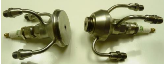
Fig. 10. Photograph of DC-excited plasma fuel nozzles, after Matveev et al [48, 89, 90].
